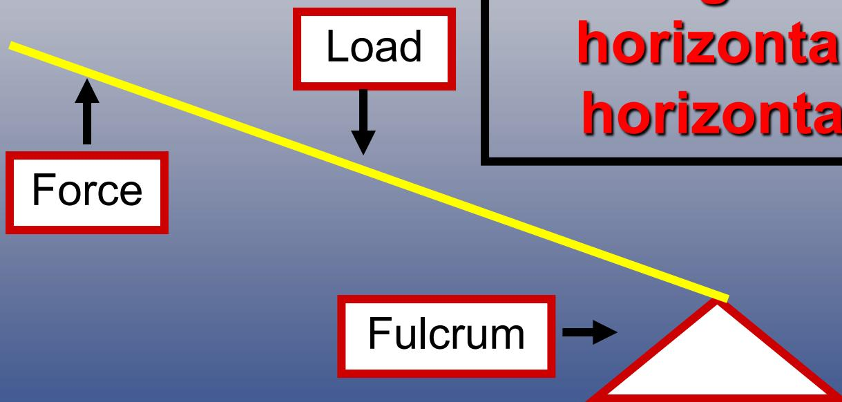
Used for advantage in moving materials on a horizontal or near-horizontal surface
